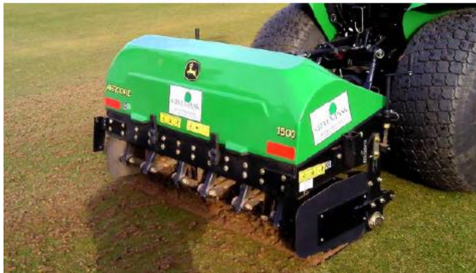
Figure 46: Air injection aerator
