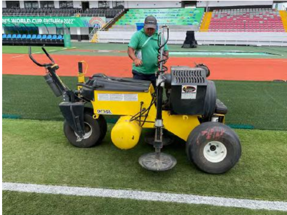
Figure 46: Air injection aerator
