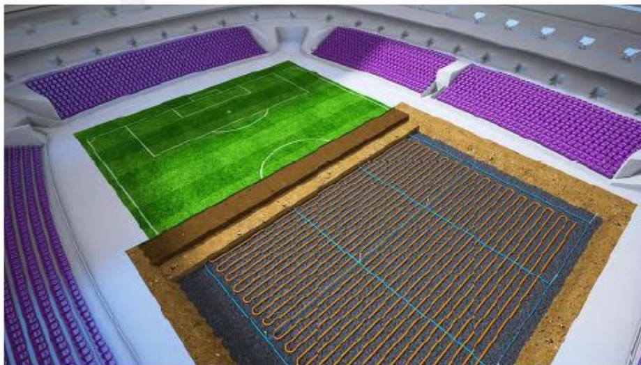
Figure 23: Conventional pipe vacuum and ventilation system
